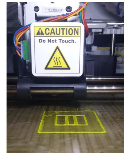
The picture on the left shows the printer in action. It takes 48 minutes to print a 60mm x 60mm x 6mm casing. The design must be bottom heavy because it prints from the bottom up.
