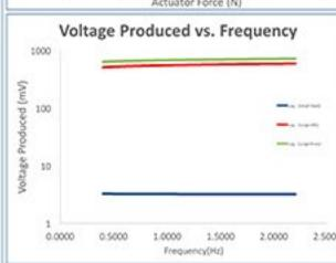
All sensors tested produced a regular voltage that was directly related to the force that the sensor experienced. In Addition, the electric potentials in all sensors were greater than anticipated, and out of the range of the lock-in in the case of the large steel sensor (over 1.0 V).
